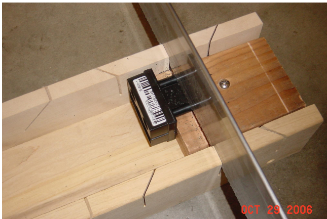
Figure 5 - Cutting 1/2" from sensor leg
