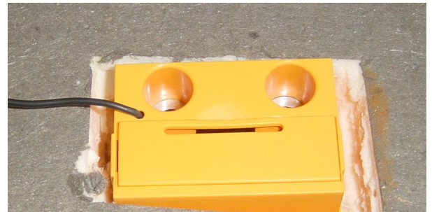
Figure 6 - Sensor In Cutout
