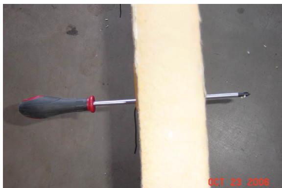
Figure 7 - Creating Pilot Hole
